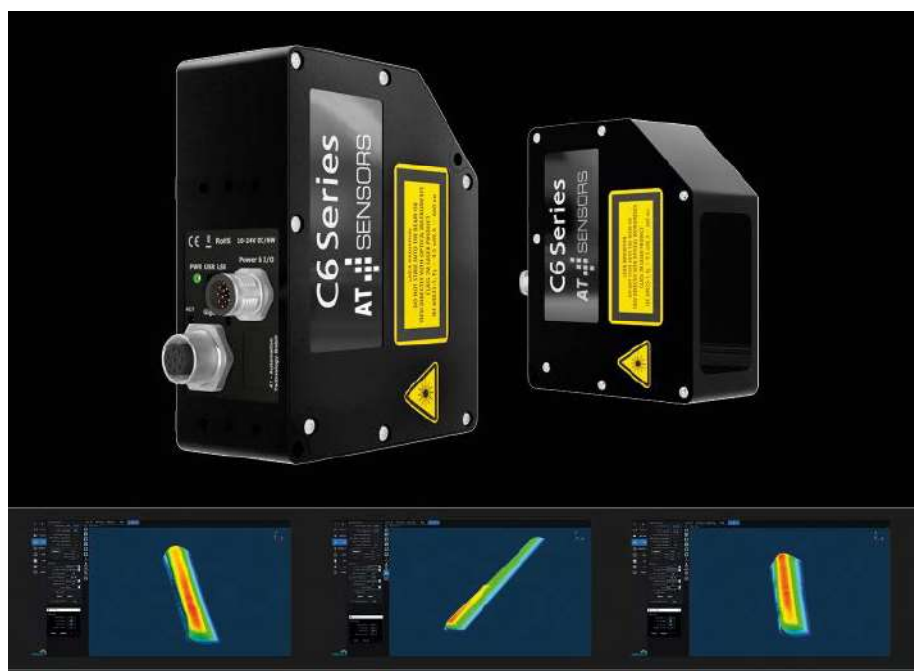
The Korean integrator GES therefore uses two AT sensors of type C6-1280CS35-7 GigE (405 nm, class 3R) for can-cap welding inspection. These offer a high resolution in X (5 \mu\text{m} ) and Z (0.2 \mu\text{m} ) as well as a profiling speed of up to 140 kHz.
