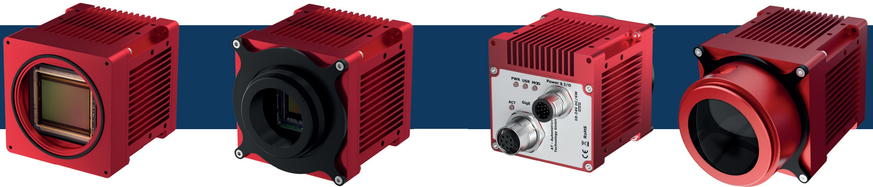
Version with Optional C-Mount Adapter
